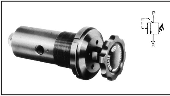
The pilot-operated relief valve is mainly used for remote control of the main circuit pressure by connecting it to the vent port (VE) of a balancing piston type relief valve. In a small-flow circuit, this type of valve can also be used as a direct acting type relief valve.
