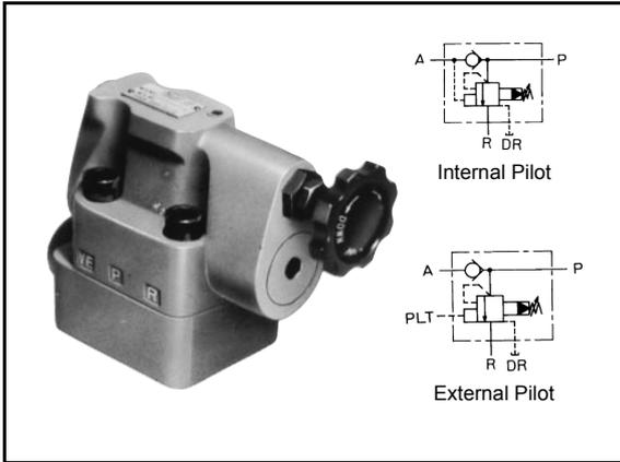
This type of valve consists of a balancing piston type unloading valve and a check valve assembled in one housing and is mainly used in accumulator circuits and circuits in which two levels of pressure (low-pressure large-volume circuit and high-pressure small-volume circuit) are handled.
